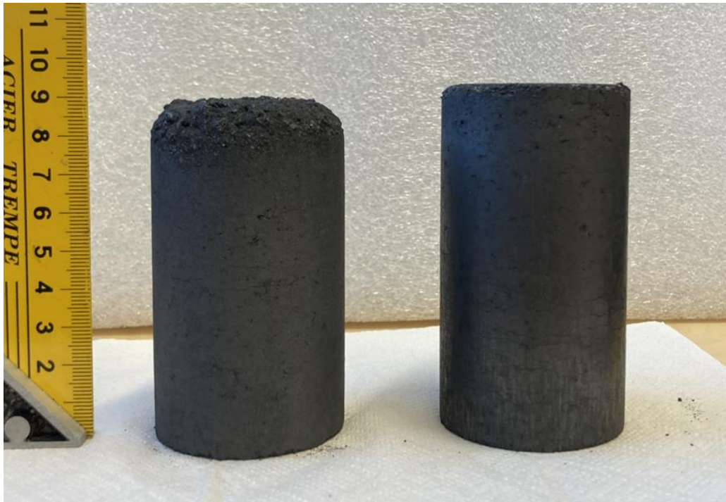
Figure 1. BP-4 (left) and CTP-4 (right) samples after baking at SINTEF.
